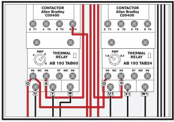
Figure 55. 220V Thermal relays.
